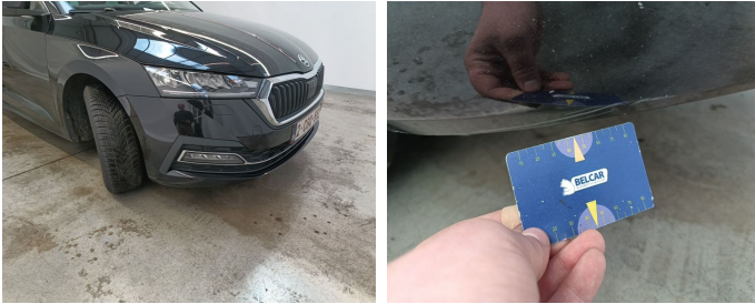
Bumper Front // Smart Repair Medium-scratch
