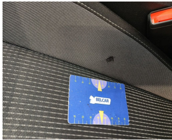
Seat Front Left / Bottom Coating / Replace-hole
