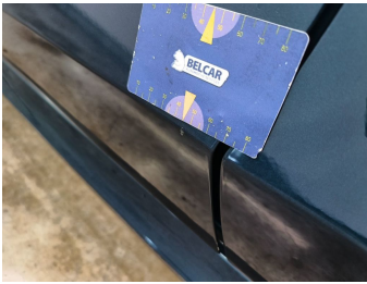
Damage within Renta-norm-scratch
