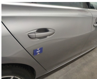
Door Rear Right // Repair & Painting-scratch + dent
