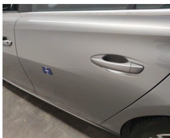
Door Rear Left // Repair & Painting-scratch + dent
