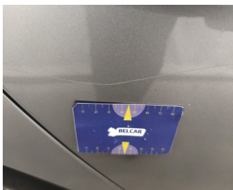
Door Rear Right // Repair & Painting-scratch + dent
