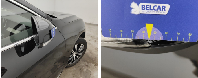
Side View Mirror Right / Direction Indicator / Replace-scratch
