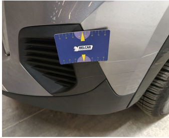
Bumper Front / Grid Left / Replace-scratch
