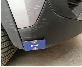
Bumper Front / Lower Cover Not Painted / Replace-scratch
