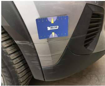
Bumper Front / Lower Cover Not Painted / Replace-scratch
