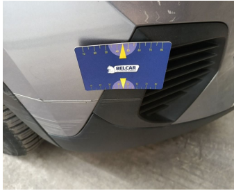
Bumper Front / Grid Right / Replace-scratch
