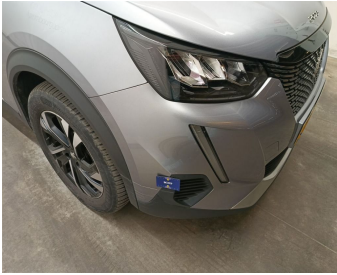
Bumper Front / Grid Right / Replace-scratch
