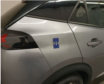
Wing Rear Right // Painting-scratch
