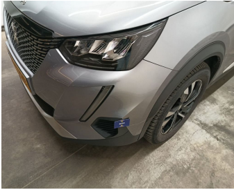
Bumper Front / Grid Left / Replace-scratch
