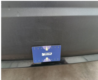
Bumper Rear / Lower Cover Not Painted / Replace-scratch
