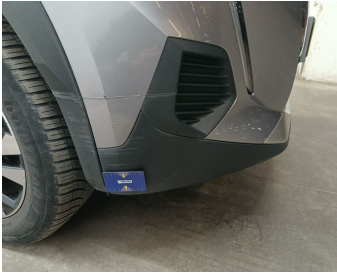
Bumper Front / Lower Cover Not Painted / Replace-scratch
