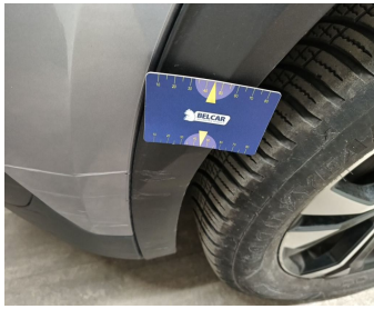
Wing Front Left / Trim / Replace-scratch
