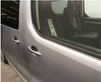
Door Front Right / Trim / Replace-scratch
