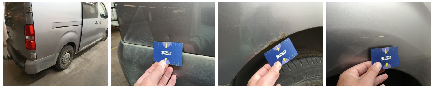
Wing Rear Left // Repair & Painting-rust
