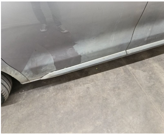
Door Front Left / Trim / Replace-cracked
