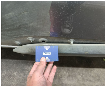
Door Front Left / Trim / Replace-cracked
