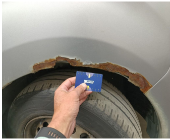
Wing Front right // Replace & Painting-rust
