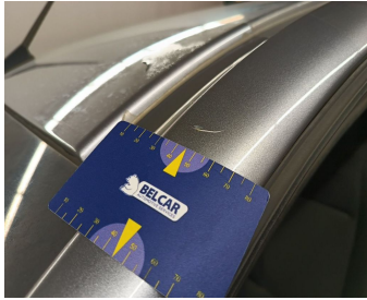
Door Front Left // Polish-Chemical reaction
