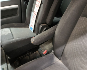
Seat Front Left / Armrest / Replace-hole
