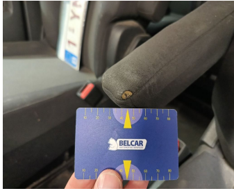
Seat Front Left / Armrest / Replace-hole
