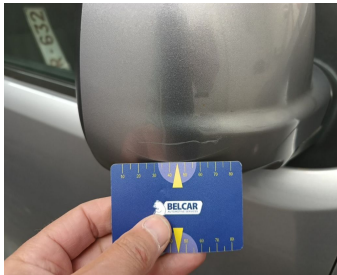
Side View Mirror Right // Painting-scratch
