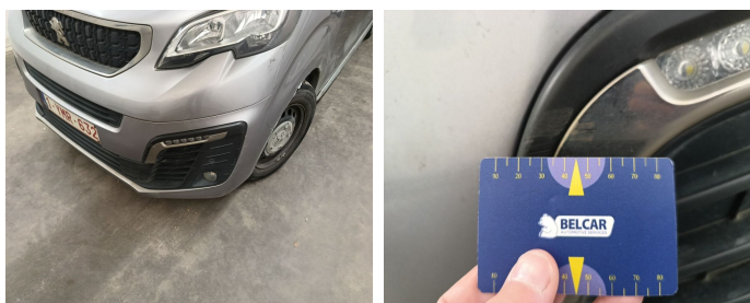
Bumper Front / Trim Left / Replace-scratch
