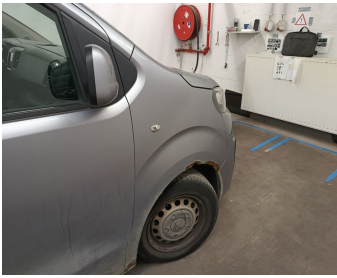
Wing Front right // Replace & Painting-rust
