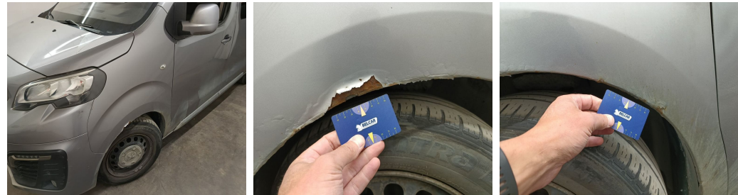
Wing Front Left // Replace & Painting-rust
