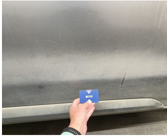
Door Front Left // Polish-Chemical reaction
