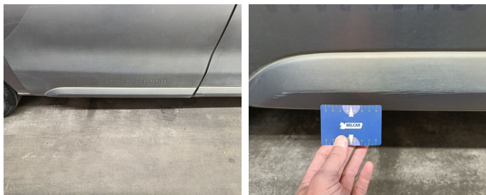
Door Rear Right / Trim / Replace-scratch
