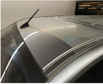
Roof // Painting-Chemical reaction
