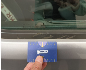
Door Front Right / Trim / Replace-scratch
