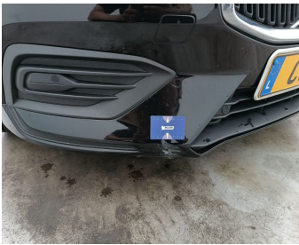
Bumper Front // Replace & Painting-cracked
