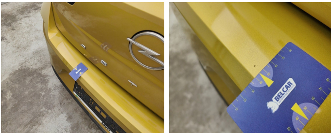
Bumper Rear // Smart Repair Medium-scratch
