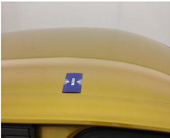
Roof // Smart Repair Medium-dent
