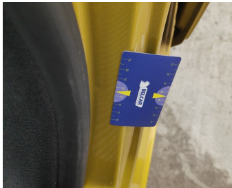
Rocker Panel Left // Smart Repair Medium-dent
