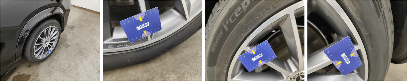
Wheel Two Tone Rear Left // Repair-scratch
