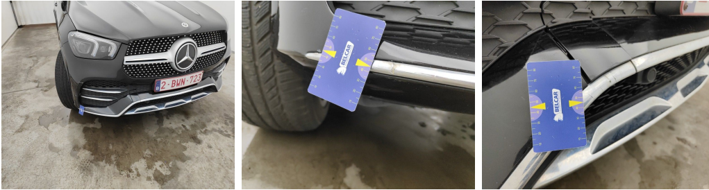
Bumper Front / Trim Right / Replace-cracked
