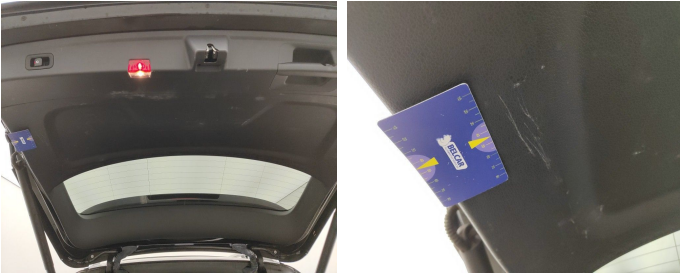
Trunk Lid Interior Coating / Complete Panel / Replace-scratch
