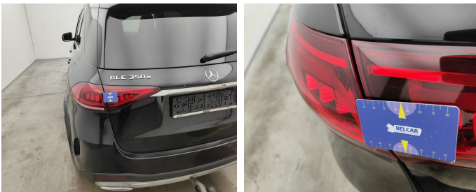
Light / Rear Left On Rear Bonnet / Replace-scratch
