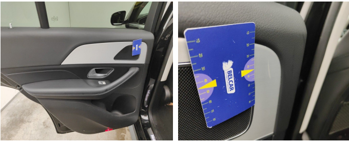
Rear Left Door Interior Coating // Repair-scratch
