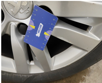
Wheel Alloy Front Right // Repair-scratch
