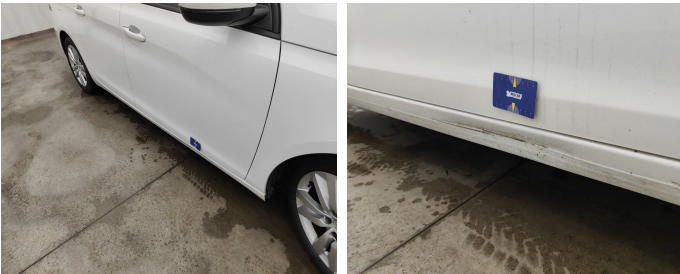
Rocker Panel Right // Repair & Painting-scratch + dent
