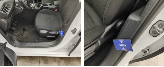
Interior / A Pillar Lower Cover / Replace-scratch
