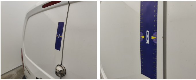
Rear Loading Door Left // Repair & Painting-scratch + dent
