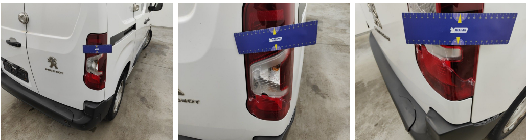
Light / Rear Right / Replace-cracked
