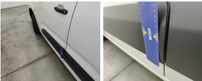
Door Front Left / Trim / Replace-scratch
