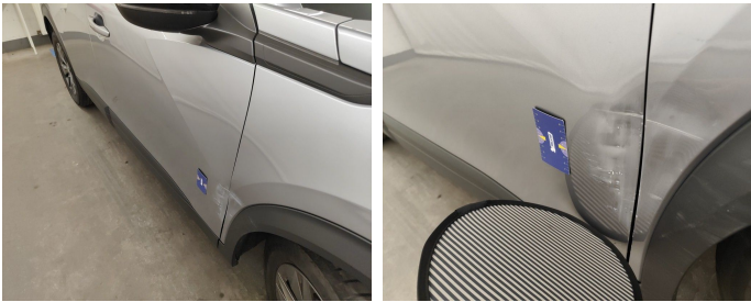
Door Front Right // Repair & Painting-scratch + dent
