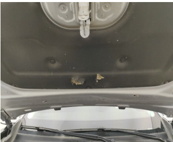
Front Bonnet / Insulation / Replace-tear
