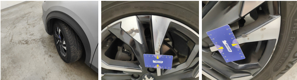
Wheel Two Tone Front Left // Repair-scratch
