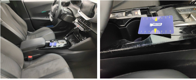
Central Console // Repair-scratch
