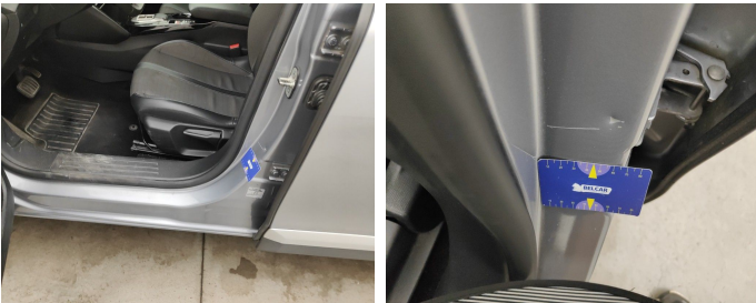
Rocker Panel Left // Smart Repair Medium-scratch + dent
