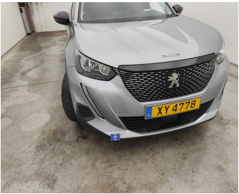
Bumper Front / Lower Cover Not Painted / Replace-scratch
