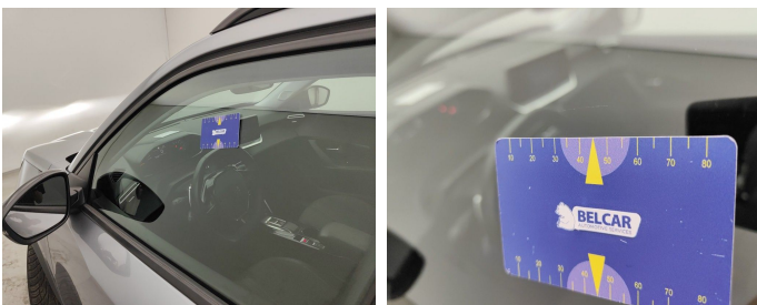
Door Front Left / Window / Replace-scratch
