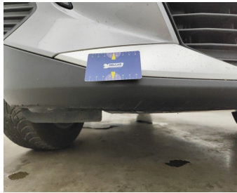
Bumper Front / Lower Cover Not Painted / Replace-scratch
