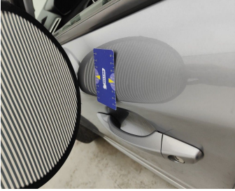
Door Front Left // Repair & Painting-scratch + dent
