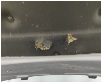
Front Bonnet / Insulation / Replace-tear
