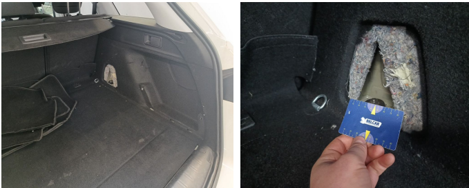
Trunk Compartment / Side Cover Right / Replace-missing
