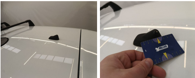
Roof / Antenna / Replace-missing
