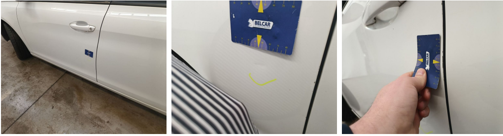
Door Front Left // Repair & Painting-scratch + dent
