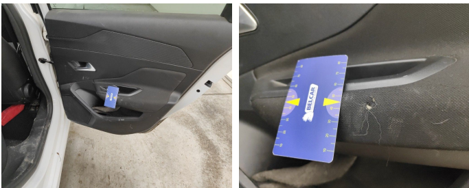
Rear Right Door Interior Coating // Repair-hole
