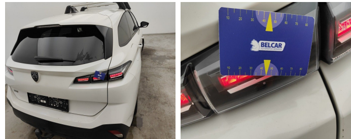
Light / Rear Right On Rear Bonnet / Replace-scratch
