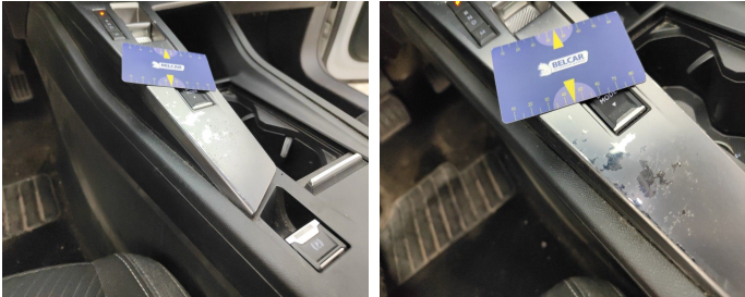
Central Console // Repair-Chipped paint
