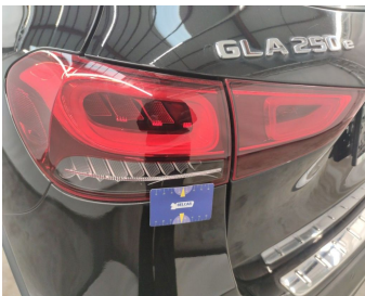
Light / Rear left / Replace-cracked
