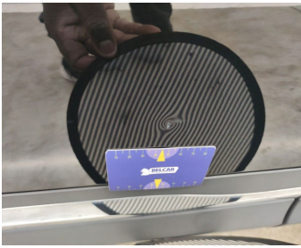
Door Rear Right // Repair & Painting-scratch + dent
