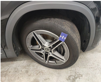
Tyre Front Right // Replace-tear
