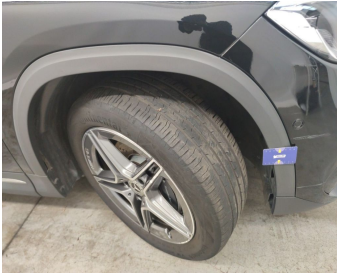
Wing Front right / Trim / Replace-scratch
