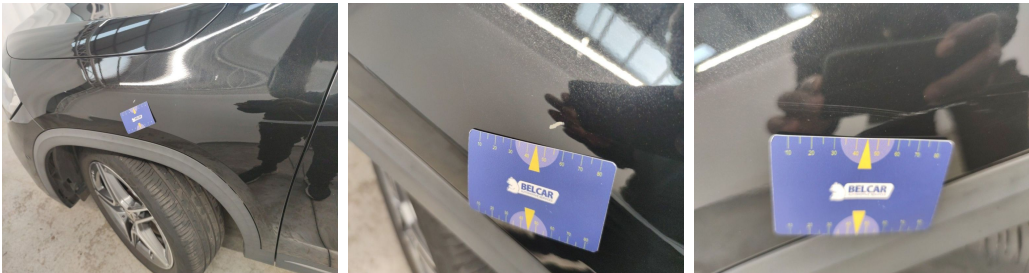
Wing Front Left // Painting-scratch
