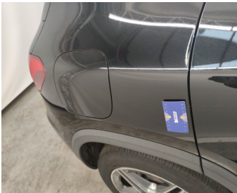
Wing Rear Right // Painting-scratch
