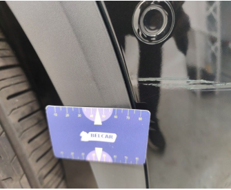
Wing Front right / Trim / Replace-scratch
