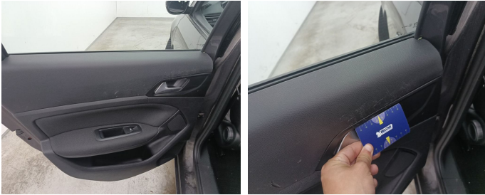
Rear Left Door Interior Coating // Replace Completely-scratch
