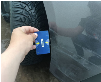
Wing Front right // Repair & Painting-scratch + dent
