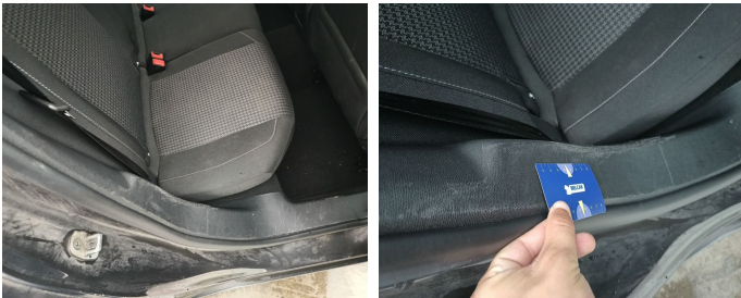
Interior / Side Cover rear Seat / Replace-scratch
