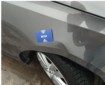
Wing Front right // Repair & Painting-scratch + dent
