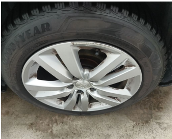
Wheel Alloy Rear Left // Repair-scratch
