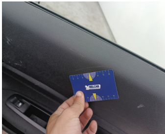
Rear Right Door Interior Coating // Replace Completely-scratch
