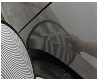
Door Rear Left // Smart Repair Small-dent
