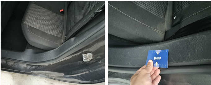
Interior / Side Cover rear Seat / Replace-scratch
