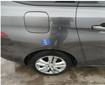
Wing Rear Right // Smart Repair Medium-scratch
