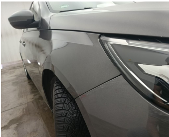
Wing Front right // Repair & Painting-scratch + dent
