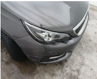
Wing Front right // Repair & Painting-scratch + dent
