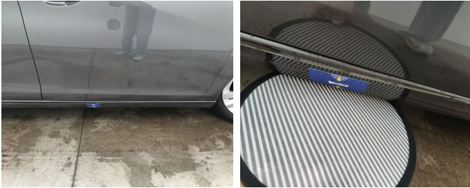
Rocker Panel Right // Repair & Painting-scratch + dent
