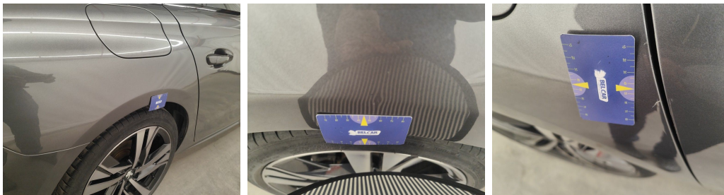
Wing Rear Right // Repair & Painting-scratch + dent
