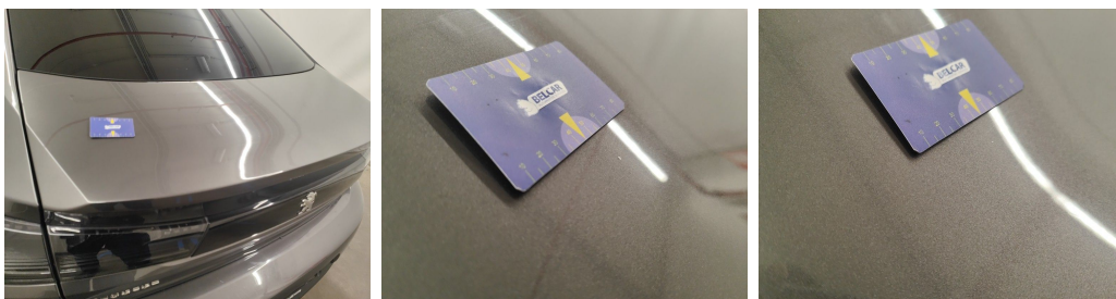
Rear Bonnet // Painting-bad repair
