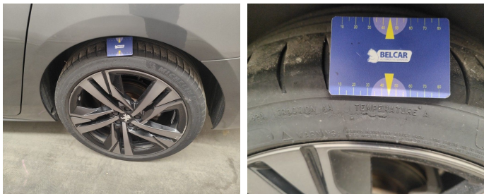
Tyre Rear Left // Replace-tear
