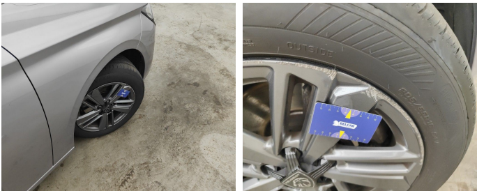
Wheel Alloy Front Right // Repair-scratch
