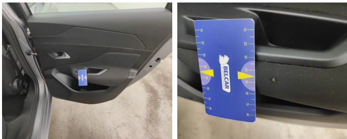
Rear Right Door Interior Coating // Repair-hole
