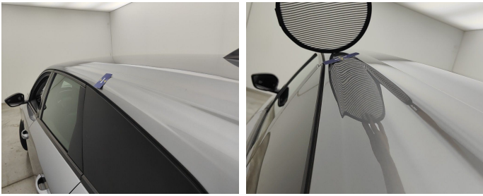
Roof // Smart Repair Medium-dent
