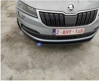
Bumper Front / Lower Cover Not Painted / Replace-scratch
