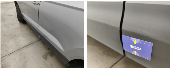
Door Rear Left / Trim / Replace-scratch
