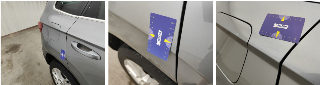
Wing Rear Right // Painting-scratch
