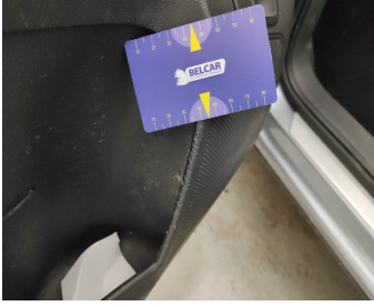
Front Left Door Interior Coating // Repair-scratch
