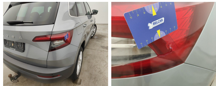
Light / Rear Right / Replace-cracked
