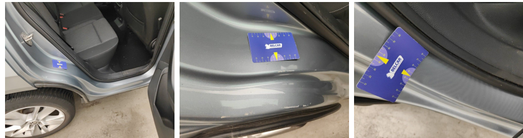
Rocker Panel Right // Smart Repair Medium-scratch + dent
