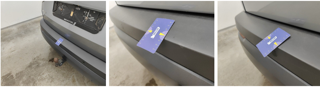
Bumper Rear / Lower Cover Not Painted / Replace-scratch
