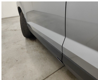
Door Front Left / Trim / Replace-scratch
