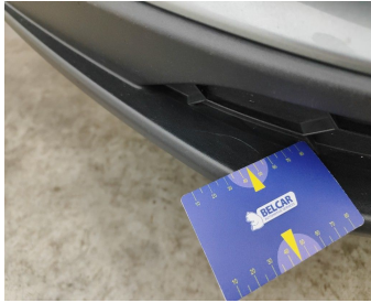
Bumper Front / Lower Cover Not Painted / Replace-scratch
