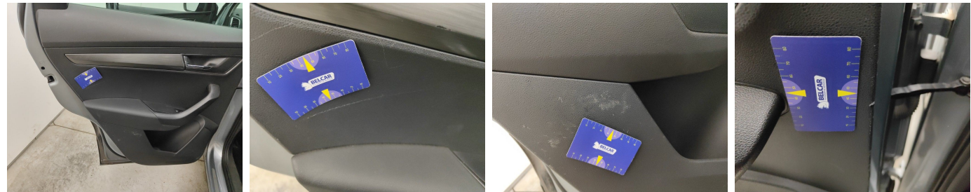
Rear Left Door Interior Coating // Repair-scratch
