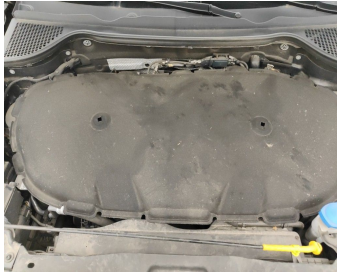
Front Bonnet / Insulation / Replace-bad position
