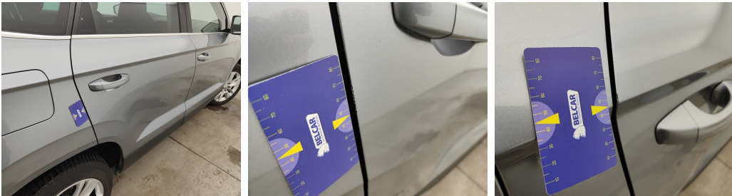
Door Rear Right // Smart Repair Small-scratch
