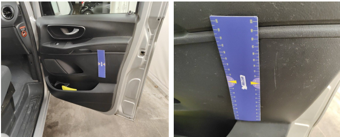
Front Right Door Interior Coating // Replace Completely-scratch
