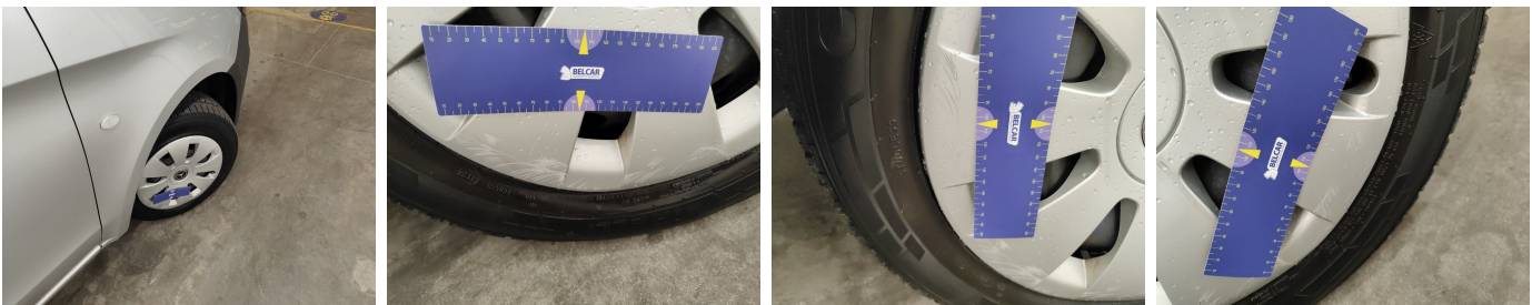
Wheel Front Right / Wheel Cover / Replace-scratch
