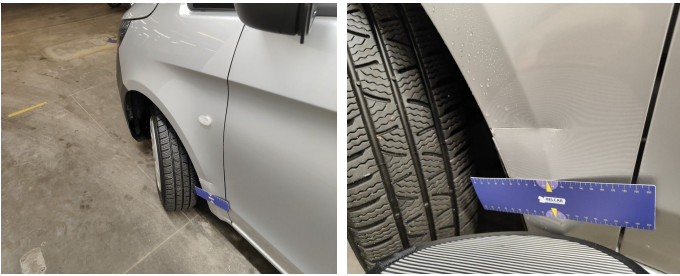
Wing Front Left // Repair & Painting-scratch + dent
