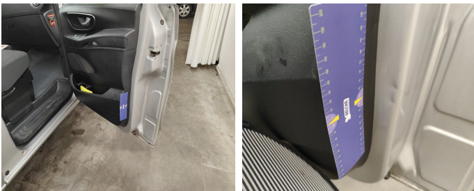
Door Front Right // Smart Repair Small-dent
