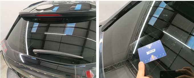
Rear Bonnet / Rear Window / Replace-scratch
