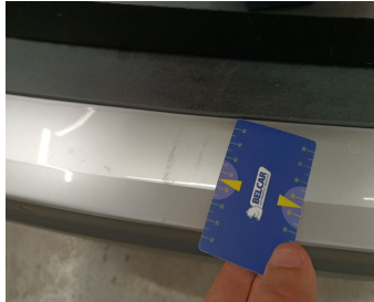
Towing Cover Rear // Replace-scratch
