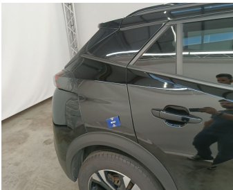
Wing Rear Right // Repair & Painting-scratch + dent
