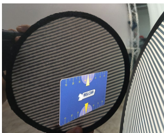
Door Front Right // Repair & Painting-bad repair
