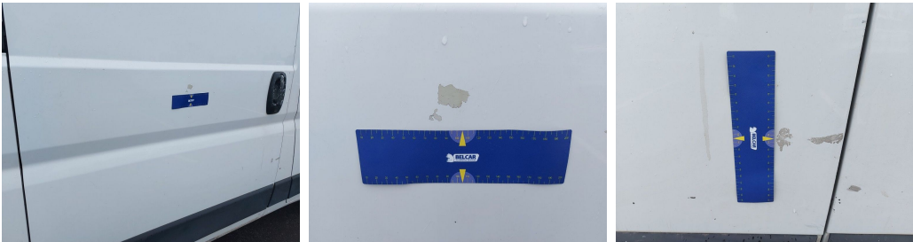
Door Rear Right // Painting-Chipped paint
