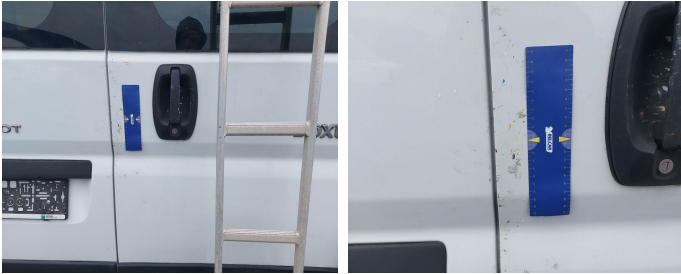
Rear Loading Door Right // Painting-scratch
