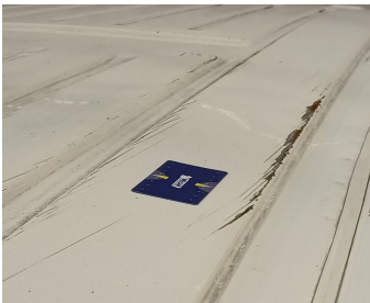
Rear Loading Door Left // Repair & Painting-scratch + dent
