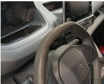
Dashboard / Steering Wheel / Replace-worn
