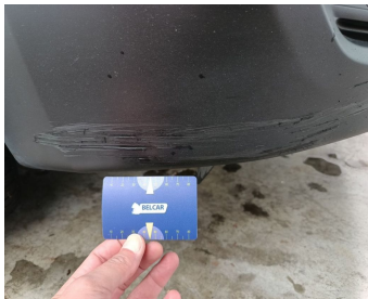
Bumper Front / Lower Cover Not Painted / Replace-scratch
