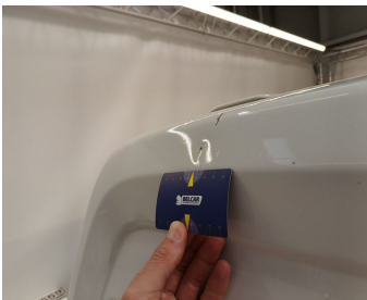
Rear Loading Door Right // Repair & Painting-scratch + dent
