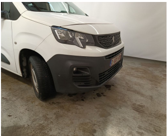
Bumper Front / Lower Cover Not Painted / Replace-scratch
