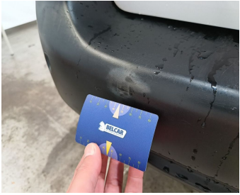
Bumper Rear // Replace without painting-scratch
