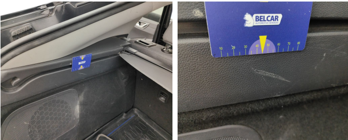
Trunk Compartment / Side Cover Left / Replace-scratch
