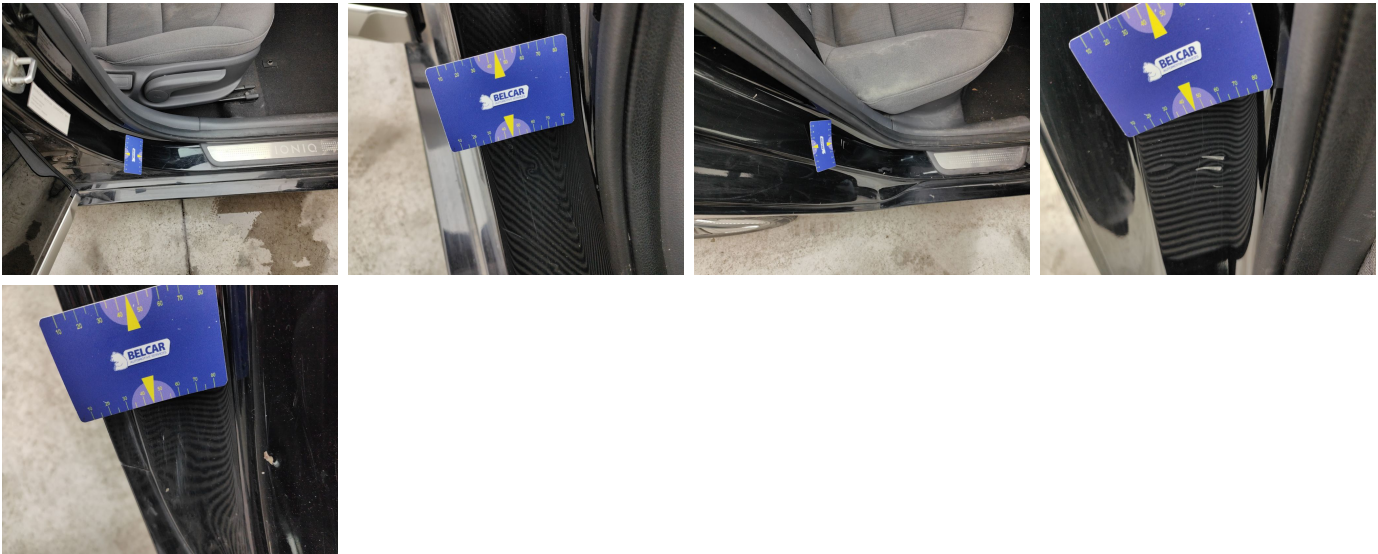
Rocker Panel Right // Smart Repair Medium-scratch + dent
