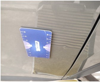
Door Front Right // Painting-scratch + dent
