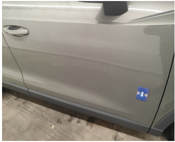
Door Front Right // Painting-scratch + dent
