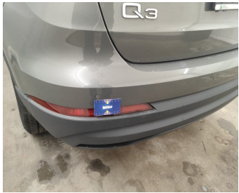
Bumper Rear // Painting-scratch + dent
