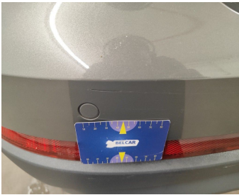
Bumper Rear // Painting-scratch + dent
