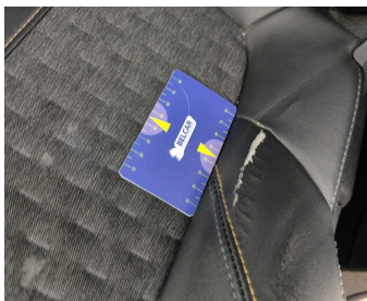
Seat Front Left / Bottom Coating / Replace-tear
