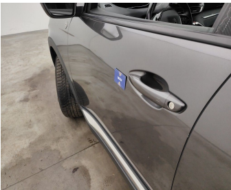
Door Front Left // Repair & Painting-scratch + dent
