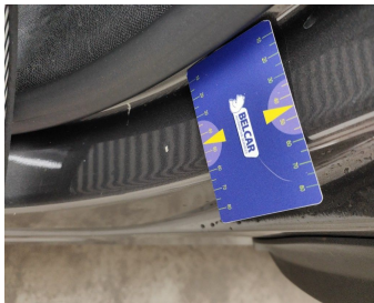
Rocker Panel Left // Smart Repair Medium-scratch + dent
