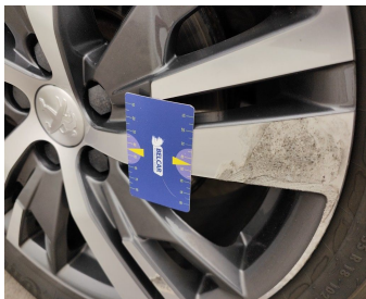
Wheel Two Tone Front Left // Repair-scratch
