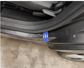
Rocker Panel Left // Smart Repair Medium-scratch + dent
