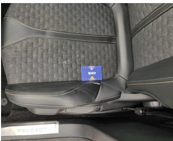
Seat Front Left / Bottom Coating / Replace-tear
