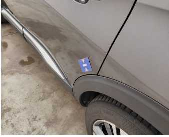
Door Rear Left // Repair & Painting-scratch + dent
