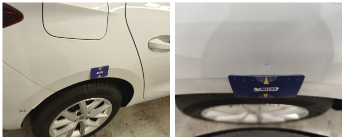
Wing Rear Right // Repair & Painting-scratch + dent
