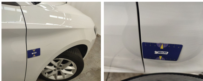
Wing Front right // Smart Repair Small-dent
