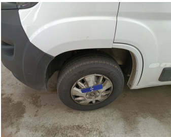
Wheel Front Left / Wheel Cover / Replace-scratch
