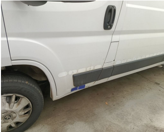
Rocker Panel Left // Repair & Painting-scratch + dent
