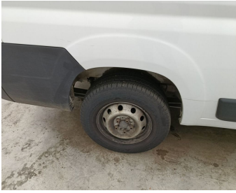
Wheel Rear Right / Wheel Cover / Replace-missing
