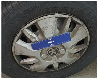
Wheel Front Left / Wheel Cover / Replace-scratch
