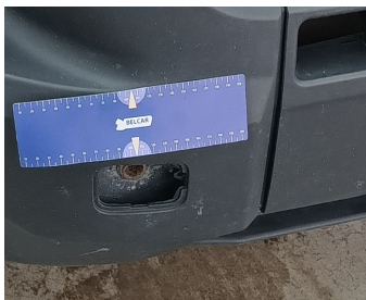
Front / Towing Cover / Replace-missing
