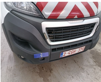
Front / Towing Cover / Replace-missing
