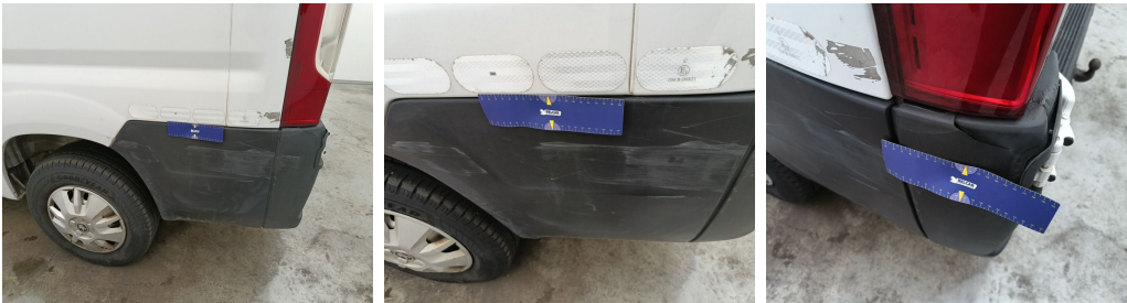
Bumper Rear // Replace without painting-cracked
