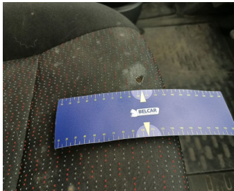
Seat Front Right / Bottom Coating / Replace-Incinerated
