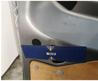
Rear Loading Door Left // Smart Repair Small-dent
