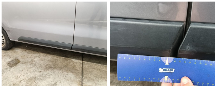
Door Rear Right / Trim / Replace-scratch
