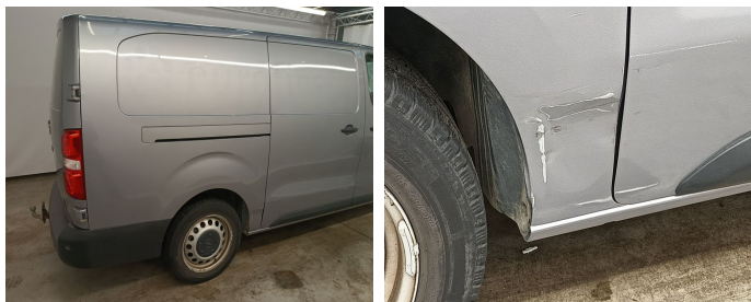
Wing Rear Right // Repair & Painting-scratch + dent
