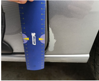
Wing Rear Left // Repair & Painting-bad repair
