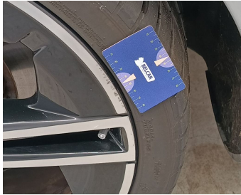
Wheel Two Tone Rear Left // Repair-scratch
