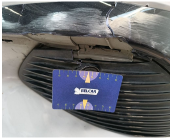
Bumper Front / Grid Left / Replace-cracked
