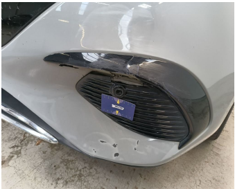
Front / Park Assist Sensor / Replace-scratch
