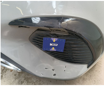
Bumper Front / Grid Left / Replace-cracked
