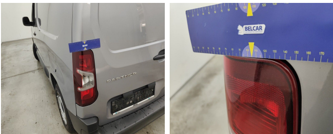
Rear Loading Door Right // Painting-bad repair
