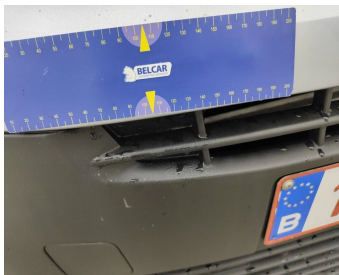
Bumper Front / Lower Cover Not Painted / Replace-Splashes
