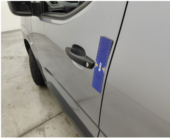
Door Front Left / Trim / Replace-scratch
