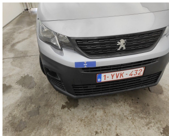
Bumper Front / Lower Cover Not Painted / Replace-Splashes
