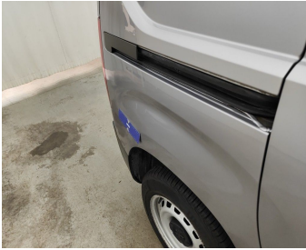
Wing Rear Right // Polish-scratch
