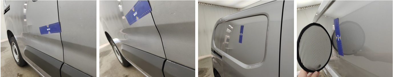
Door Rear Right // Repair & Painting-dent
