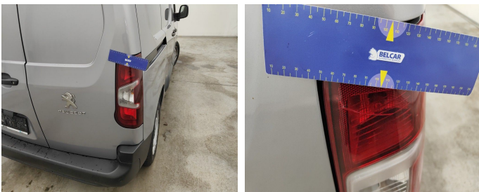
Light / Rear Right / Replace-cracked
