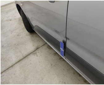
Door Front Left / Trim / Replace-scratch
