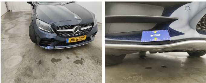
Bumper Front / Trim Right / Replace-scratch
