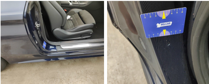
Rocker Panel Right // Smart Repair Medium-scratch + dent
