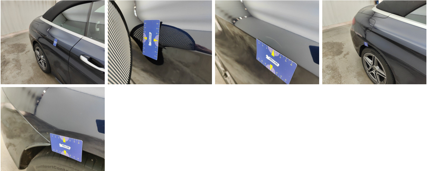
Wing Rear Right // Repair & Painting-scratch + dent
