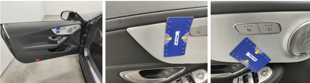
Front Left Door Interior Coating // Replace Completely-scratch
