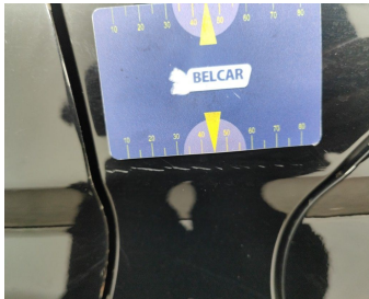
Rear Left Door Interior Coating / Grid Loudspeaker / Replace-scratch
