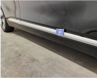
Rocker Panel Left // Smart Repair Medium-scratch + dent
