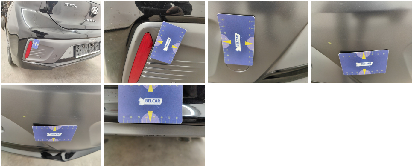
Bumper Rear / Lower Cover Not Painted / Replace-scratch
