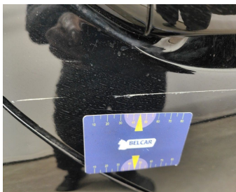
Door Rear Left // Smart Repair Medium-scratch
