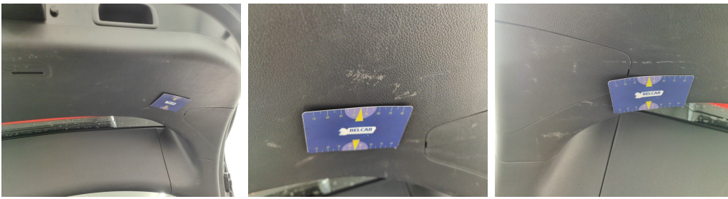
Trunk Lid Interior Coating / Complete Panel / Replace-scratch
