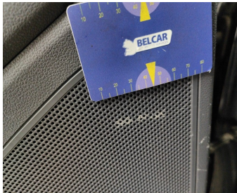
Rear Left Door Interior Coating / Grid Loudspeaker / Replace-scratch
