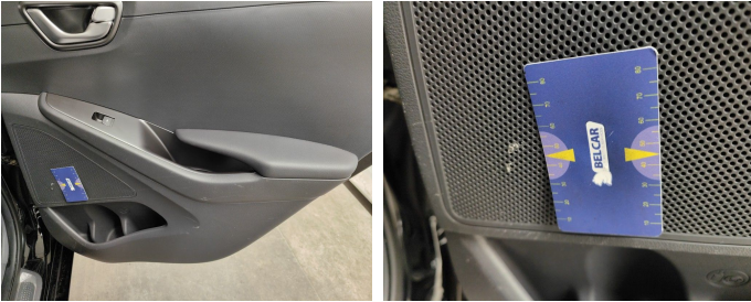
Rear Right Door Interior Coating / Grid Loudspeaker / Replace-scratch
