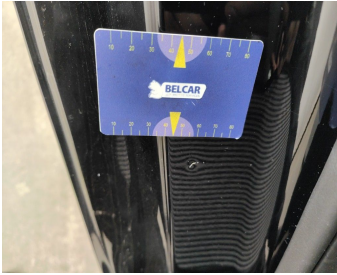
Rocker Panel Right // Repair & Painting-scratch + dent
