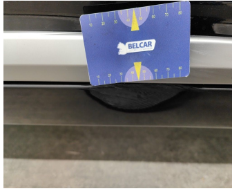
Rocker Panel Left // Smart Repair Medium-scratch + dent
