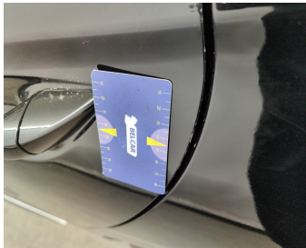
Door Rear Left // Smart Repair Medium-scratch
