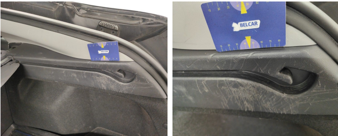
Trunk Compartment / Side Cover Right / Replace-scratch
