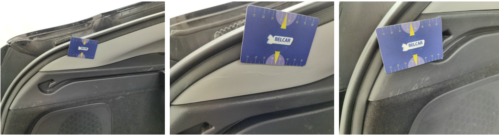
Trunk Compartment / Side Cover Left / Replace-scratch
