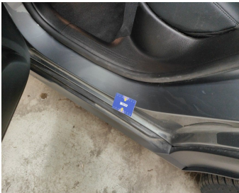
Rocker Panel Left // Smart Repair Medium-scratch
