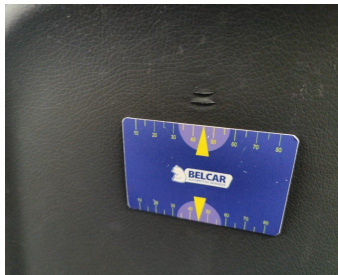
Rocker Panel Left // Smart Repair Medium-scratch
