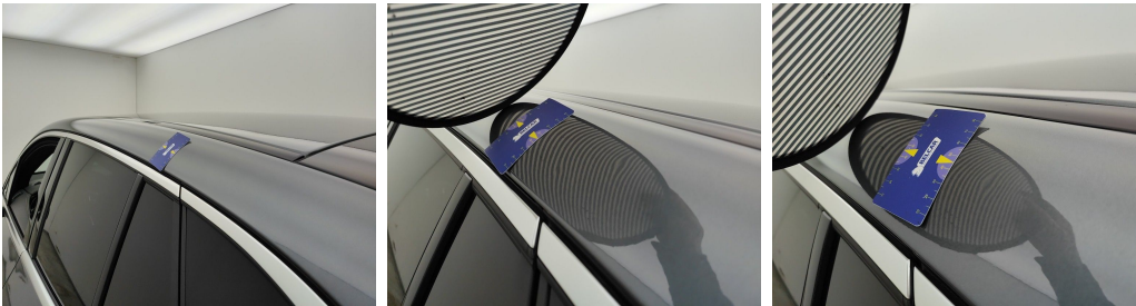
Roof // Smart Repair Medium-dent
