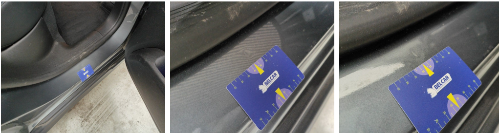
Rocker Panel Right // Smart Repair Medium-scratch + dent
