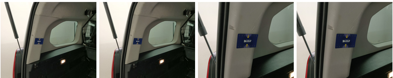
Trunk Compartment / Side Cover Left / Replace-scratch
