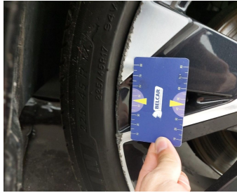
Wheel Two Tone Front Right // Repair-scratch
