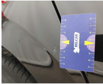
Door Rear Left // Repair & Painting-scratch + dent
