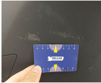
Trunk Lid Interior Coating / Complete Panel / Replace-scratch
