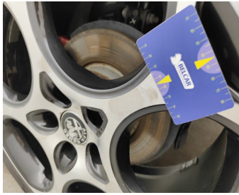
Wheel Two Tone Front Left // Repair-scratch
