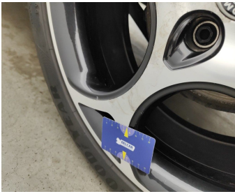
Wheel Two Tone Rear Left // Repair-scratch
