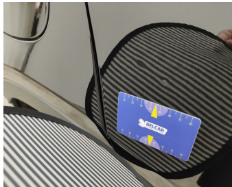
Door Rear Right // Repair & Painting-scratch + dent
