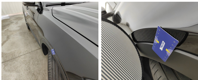
Wing Front right // Painting-bad repair
