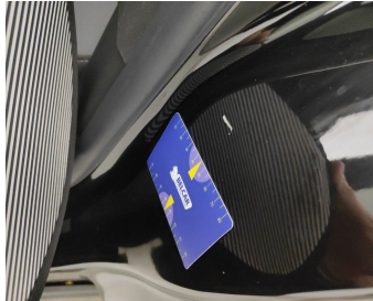
Rocker Panel Left // Smart Repair Medium-scratch + dent
