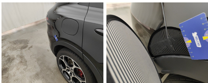
Wing Rear Right // Repair & Painting-scratch + dent
