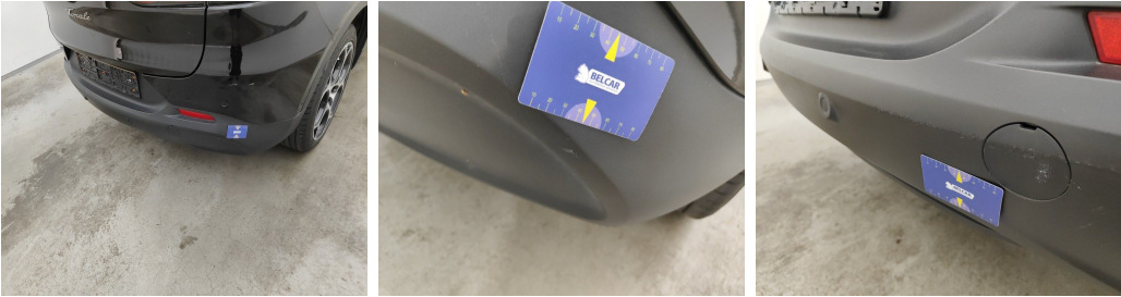
Bumper Rear / Lower Cover Not Painted / Replace-scratch
