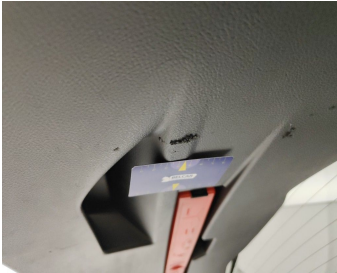
Trunk Lid Interior Coating / Complete Panel / Replace-scratch
