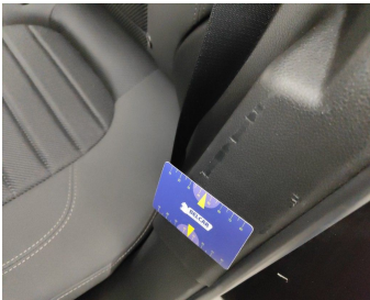
Rear Right Door Interior Coating // Replace Completely-scratch
