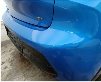
Bumper Rear / Spoiler / Replace-scratch
