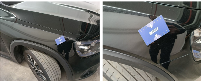
Wing Front right // Painting-stone chipping
