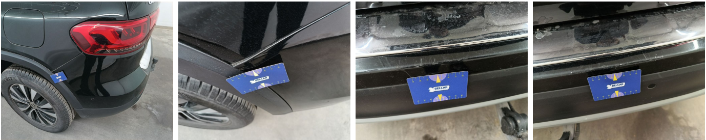
Bumper Rear // Repair & Painting-scratch + dent
