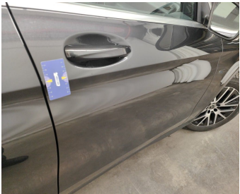
Door Front Right // Painting-scratch + dent
