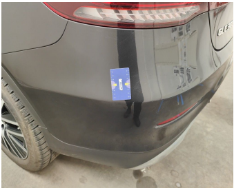
Bumper Rear // Painting-bad repair
