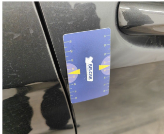
Door Front Right // Painting-scratch + dent
