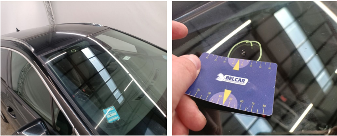
Windshield // Replace-glass damage
