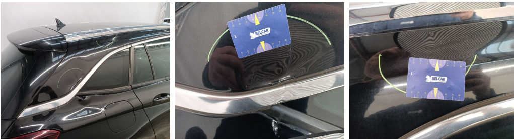
Roof // Repair & Painting-scratch + dent
