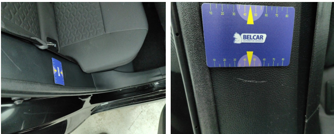
Interior / Side Cover rear Seat / Replace-scratch
