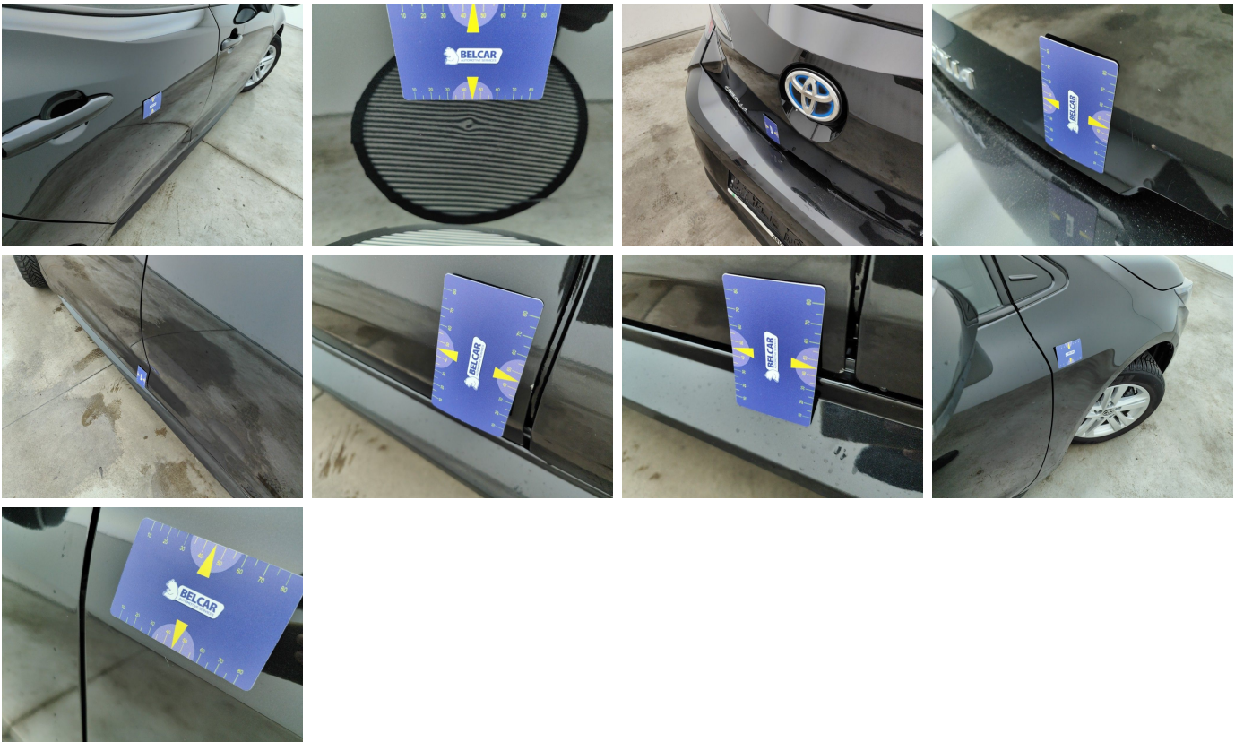
Damage within Renta-norm-dent
