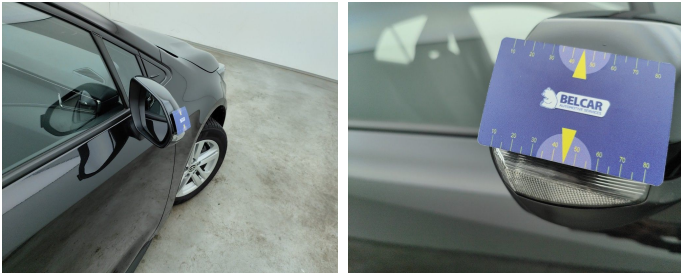
Side View Mirror Right / Direction Indicator / Replace-scratch
