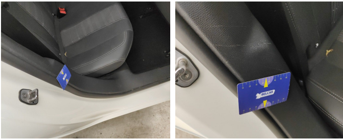
Interior / Side Cover rear Seat / Replace-scratch
