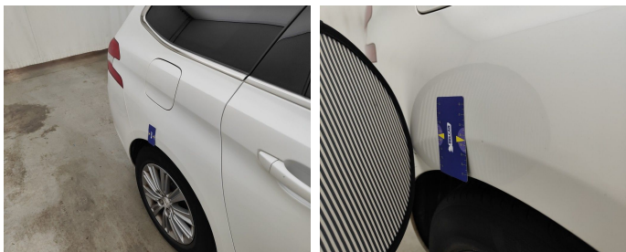
Wing Rear Right // Repair & Painting-scratch + dent
