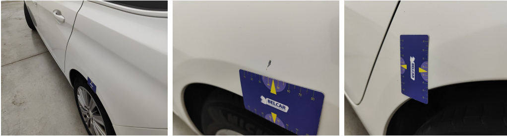
Wing Rear Left // Painting-Chipped paint
