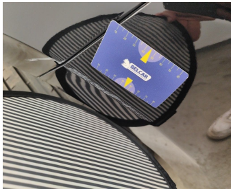
Wing Rear Left // Repair & Painting-scratch + dent
