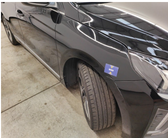
Wing Front right // Repair & Painting-scratch + dent
