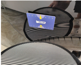
Wing Rear Right // Smart Repair Small-dent
