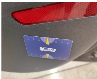
Front Right Door Interior Coating // Replace Completely-scratch
