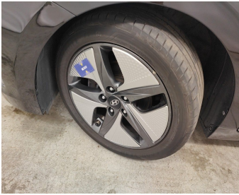
Wheel Front Left / Wheel Cover / Replace-scratch
