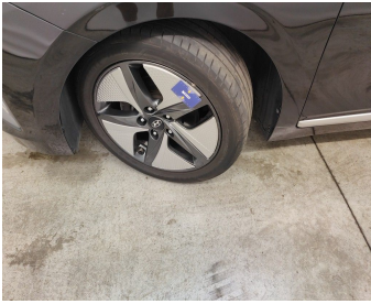
Wheel Alloy Front Left // Replace-scratch + dent
