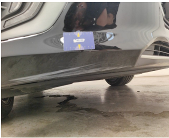
Bumper Front // Repair & Painting-scratch + dent
