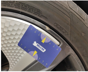
Wheel Alloy Front Left // Replace-scratch + dent
