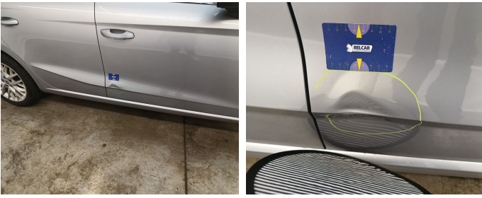
Door Front Right // Repair & Painting-scratch + dent
