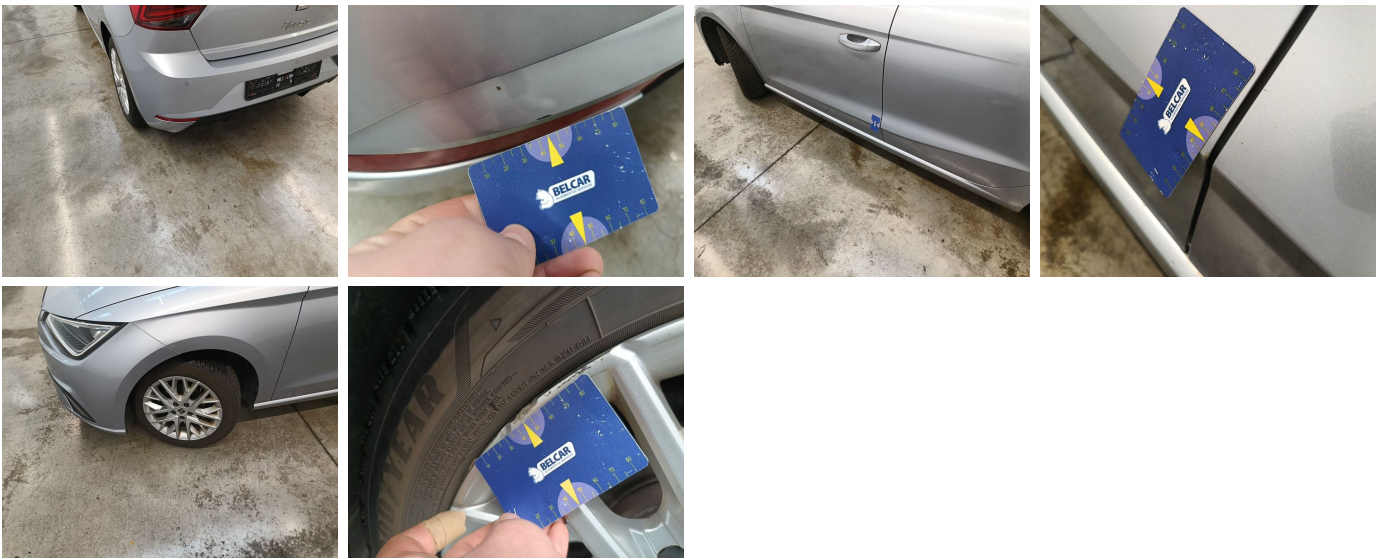
Damage within Renta-norm-scratch
