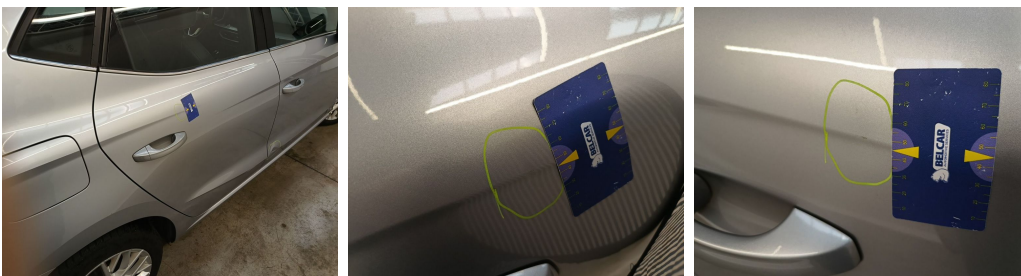
Door Rear Right // Repair & Painting-scratch + dent
