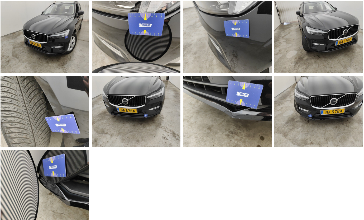
Bumper Front // Repair & Painting-scratch + dent
