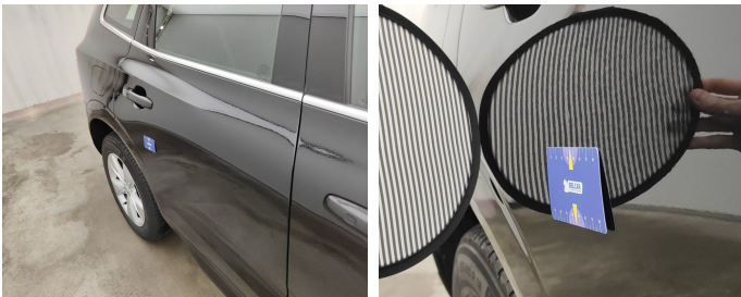
Door Rear Right // Repair & Painting-scratch + dent
