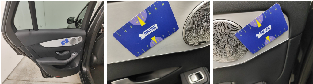
Rear Left Door Interior Coating // Repair-scratch
