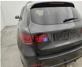
Light / Rear Left On Rear Bonnet / Replace-scratch
