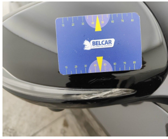
Side View Mirror Right // Painting-scratch
