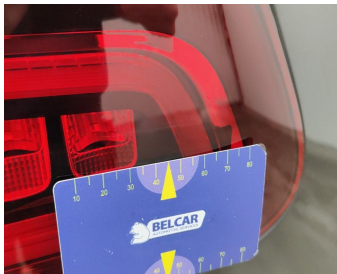
Light / Rear Left On Rear Bonnet / Replace-scratch
