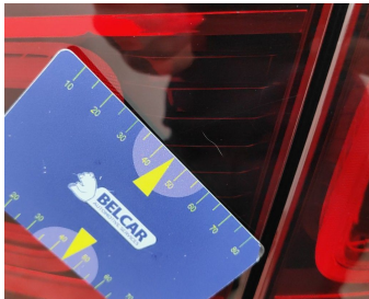
Light / Rear Right On Rear Bonnet / Replace-scratch
