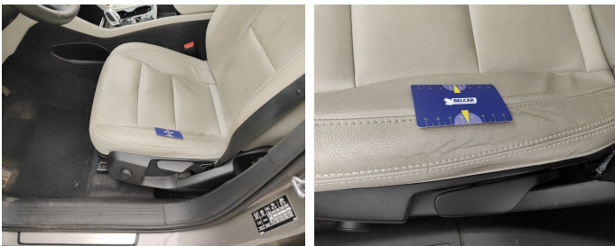
Seat Front Left / Bottom Coating / Replace-worn
