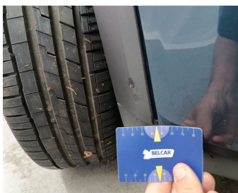
Wing Front right / Trim / Replace-bad position
