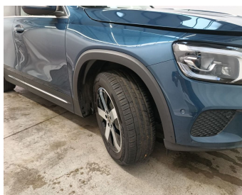
Wing Front right / Trim / Replace-bad position
